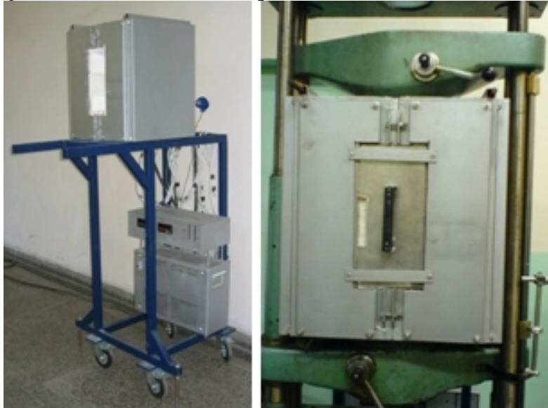
Fig.1 Heating module for material strength testing at increased temperatures
