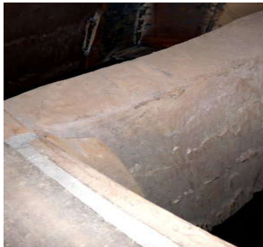
fig.7 Laser-Hybrid reconditioned pallets
