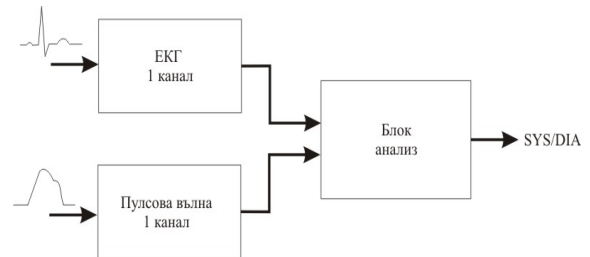
fig. 3. Block diagram for time measurement for AKH
