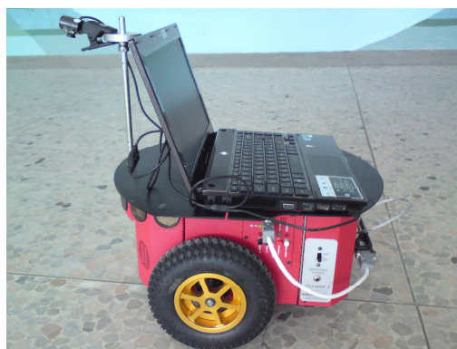
fig.1 The differential-drive wheeled mobile robot Pioneer-3DX equipped with a camera
