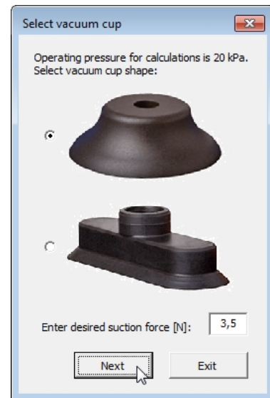
Fig.5 Selection for vacuum cup shape and lifting force
