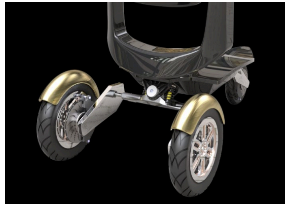
Fig.8 Extension ribs, connecting the channel truck and the wheel hub.
