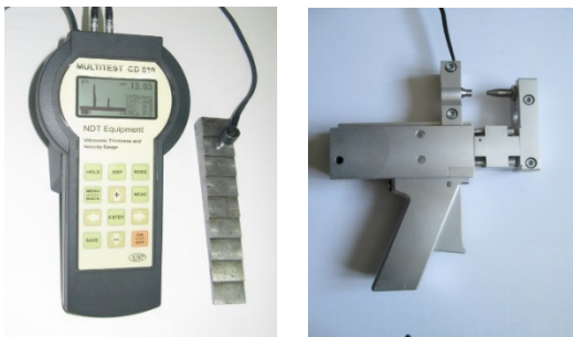
Fig.1: a) Ultrasound device MULTITEST CD 010; b) Measuring pliers DK100.
