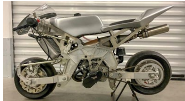
fig.3 Vehicle with a Hub-center steering.
